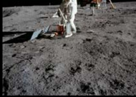
Buzz Aldrin placing one of the seismometers left on the Moon during the Apollo Missions between 1969-1972.
